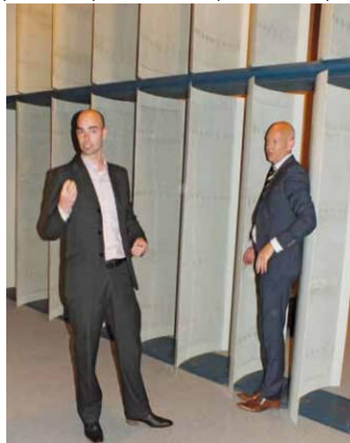
The angled vanes guide the wind in the right direction and attenuate the fan sound so a clean and silent air flow is created in the wind tunnel.
