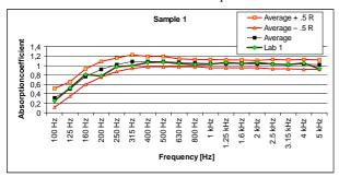
Figure 6: Illustration of the average and spread  $(\pm \frac{1}{2}R)$  of sample 1 and the indvidual result of one laboratory (green).
