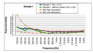
Figure 2: Reproducibility of sample 1 according to [1b]. For 13 labs (blue line) and for 9 labs (green line). Also indicated are the indications for the Reproducibility of a high and a low absorptive sample [1a].
