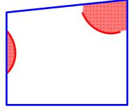
Figure 5: Illustration of the shielding by a suspended diffuser (upper right) and the more defined situation for volume diffusers (left).
