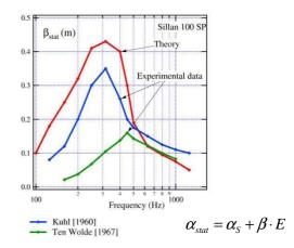
Figure 4: The edge effect: the absorption of a finite sample is composed of the absorption of an infinite sample  $(\alpha_{r})$  and a factor  $\beta$  multiplied with the relative
