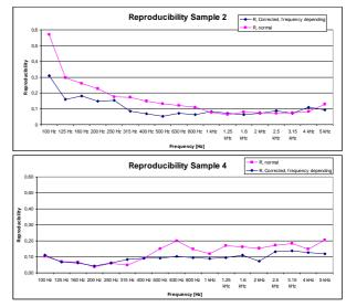
Figure 7: The effect of correcting for the reference absorber (sample 1) on the Repoducibility of sample 2 (upper graph) and sample 4 (lower graph).
